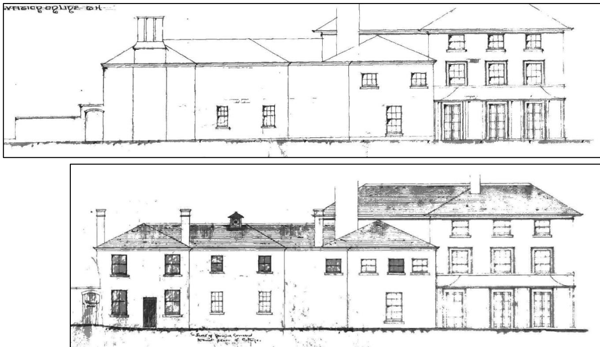
Figures 9 & 10: As Existing and Proposed' drawings prepared for W Hatton Esq c. 1870 by Bidlake & Fleeming: West elevation showing the main house with loggia and a two storey west wing. The proposals incorporated a Billiards Room to the first floor, denoted by a small clock turret or louvered ventilator to the roofline. Proposed alterations are highlighted in grey.
