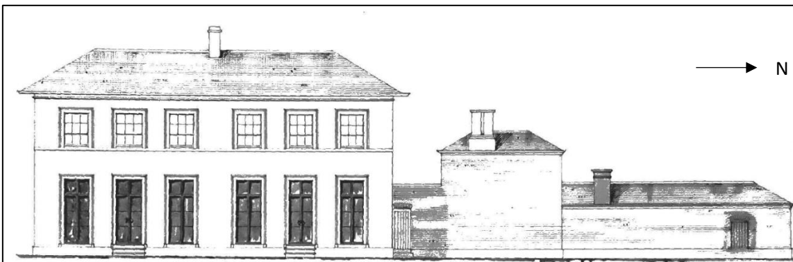
Figure 6: Drawings for W Hatton Esq c. 1870 by Bidlake & Fleeming: 'proposed' East elevation showing the two storey laundry/kitchen wing to the north of the principal house and casement windows and doors to the ground floor.
