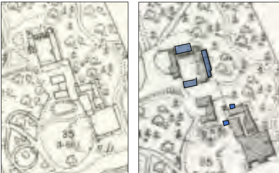
Figure 17: (Right) Ordnance Survey mapping of 1903 showing additions to Bottom yard (in blue), in comparison with (Right) the 1887 map (Left) (Ordnance Survey, 1887 and 1903). Reproduced with the permission of the National Library of Scotland
