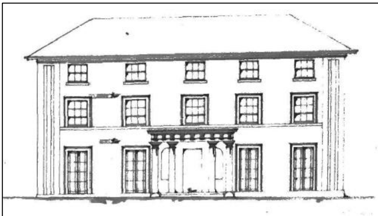
Figure 5: Drawings for W Hatton Esq c. 1870 by Bidlake & Fleeming. Main (south) elevation of the Principal House showing the house in its original form of c1814 and casement/French windows apparently in situ by this date
