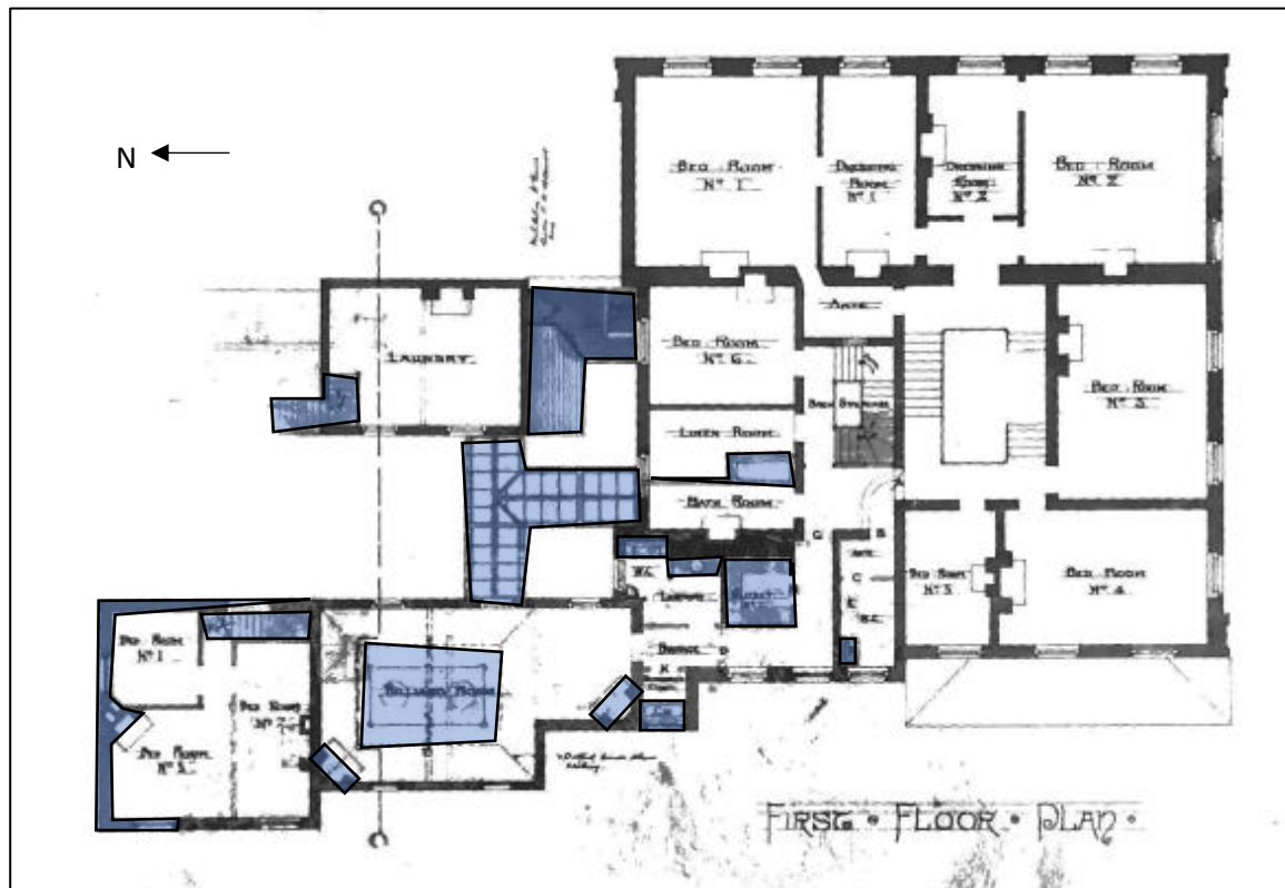
Figure 14: Drawings prepared for W Hatton Esq c. 1870 by Bidlake & Fleeming: First Floor Plan. The proposed elements have been highlighted in blue
